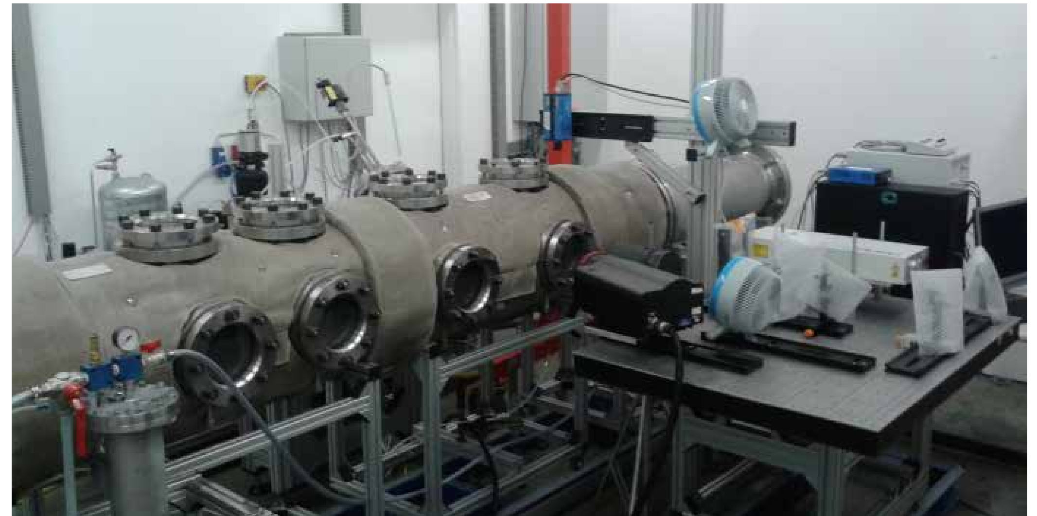
Hot exhaust gas flow rig for investigation of urea injection, evaporation and mixing
