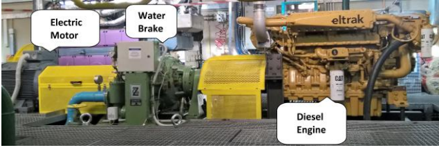
Fig. 1. The hybrid diesel-electric test bed (HIPPO-1) at LME.
