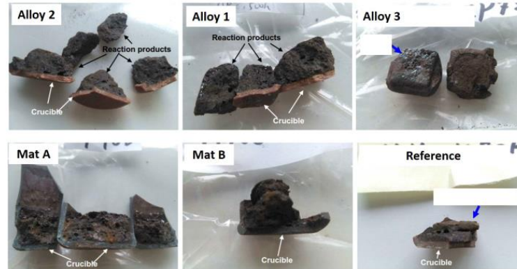
Samples of the investigated materials after high temperature corrosion testing in a vanadium containing salt solution.
