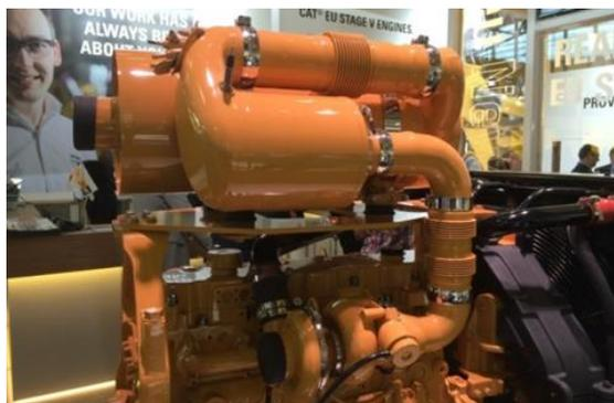
**Figure 13.** Cat C9.3B heavy-duty engine with a compact engine-mounted after-treatment system (Gehm et al. 2016b.)
