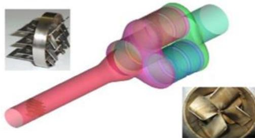
**Figure 7.** Schematics of the baseline SCR system design for large marine engine. Top-left: Two-stage mixer; bottom-right: Butterfly mixer (modified: Zheng et al 2014).
