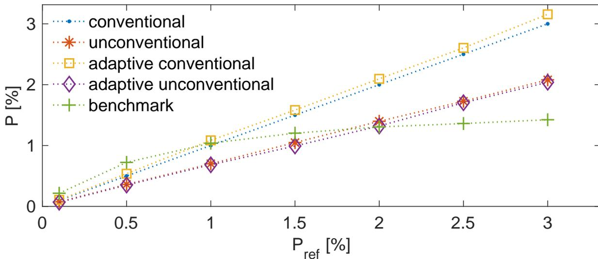
Figure 7. Actual knock rate ( $P$ ) vs. reference probability ( $P_{ref}$ ). The other parameters are equal to those listed in Table I.
