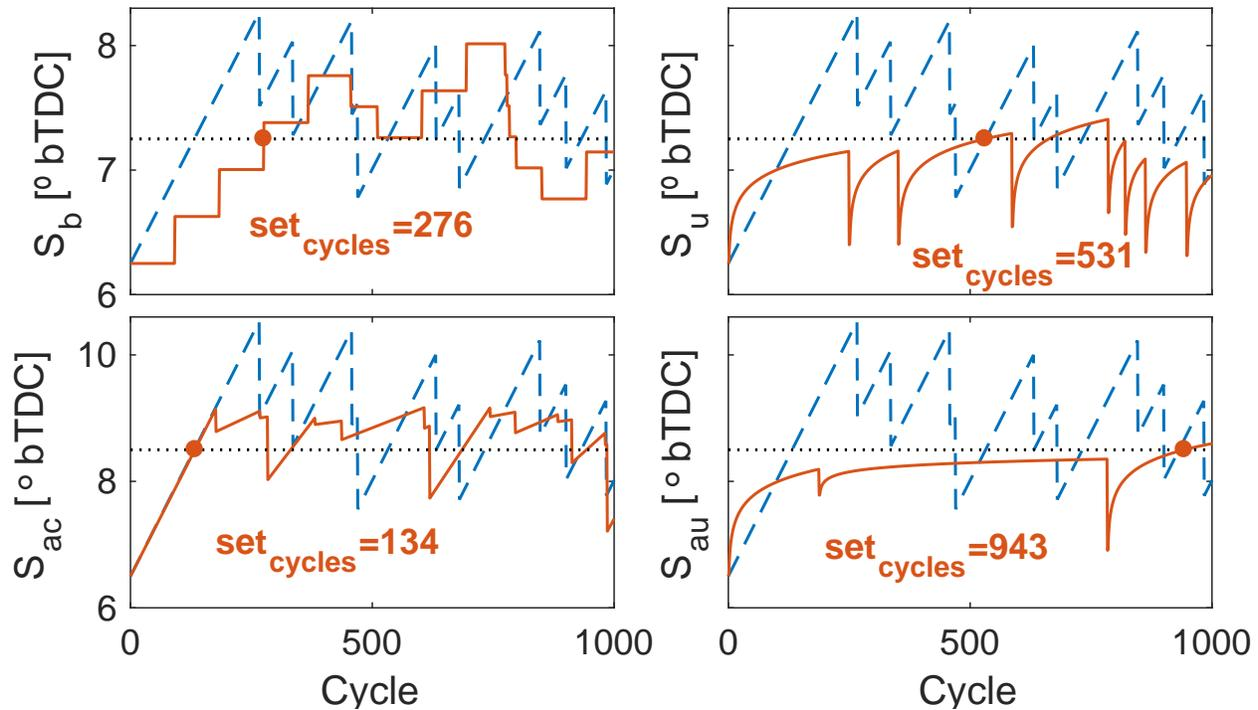
Figure 11. Evolution of the spark timing starting from retarded condition. In each subplot the conventional controller (dashed line) is compared with the benchmark (top left), the unconventional (top right), the adaptive conventional (bottom left), and the adaptive unconventional controllers (bottom right).
