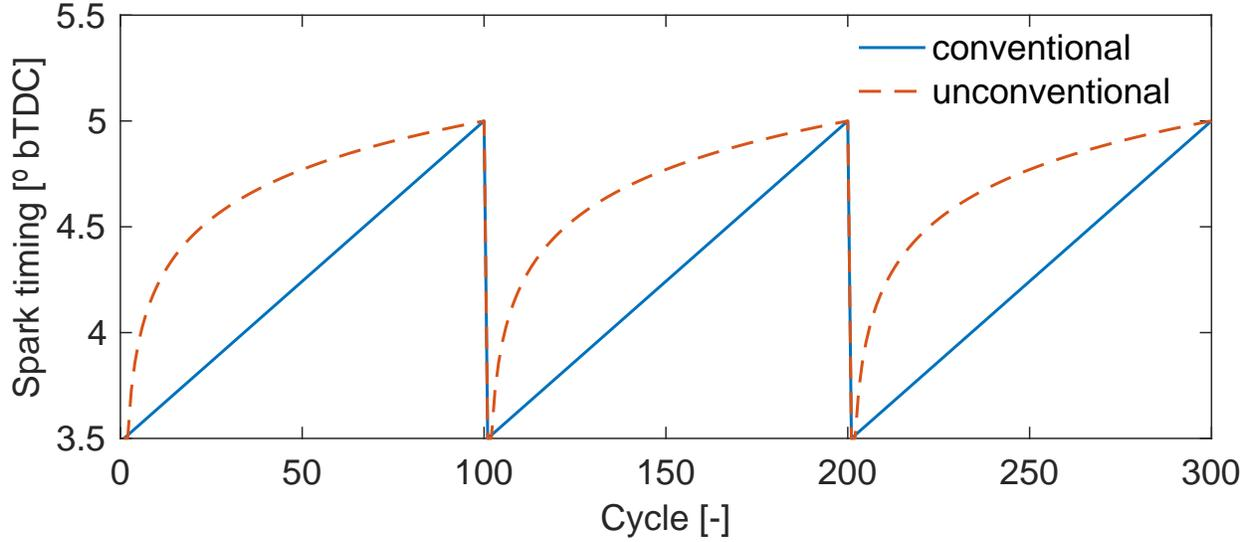
Figure 4. Unconventional vs. conventional controller evolution.  $K_{ret} = 1.5^\circ$ ,  $P_{ref} = 1\%$  and  $N_{ref} = 100$  cycles.
