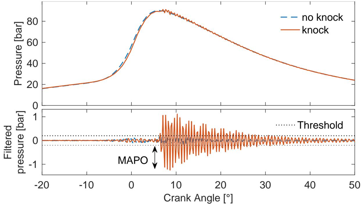
Figure 1. Raw and band-filtered pressure traces and MAPO index for a knocking and a non-knocking cycle.
