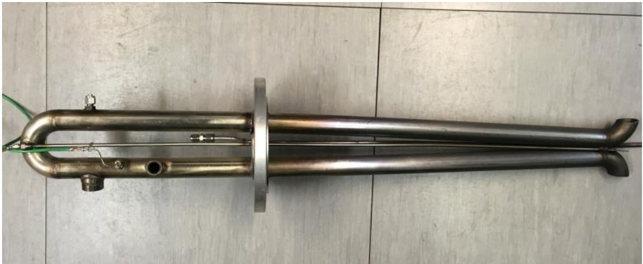
Figure 18. NH 3 sensor installation probe used in ship trial 3.
