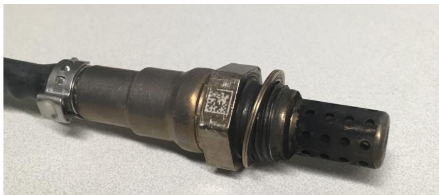
Figure 40. NH 3 sensor after the trial 3, only minor soot contamination on the sensor tip.
