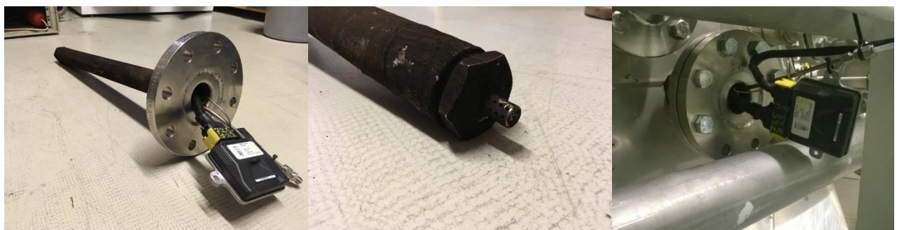
Figure 16. On the left the sensor installation probe, in the middle sensor tip at the end of the probe, on the right sensor installed in the exhaust line.
