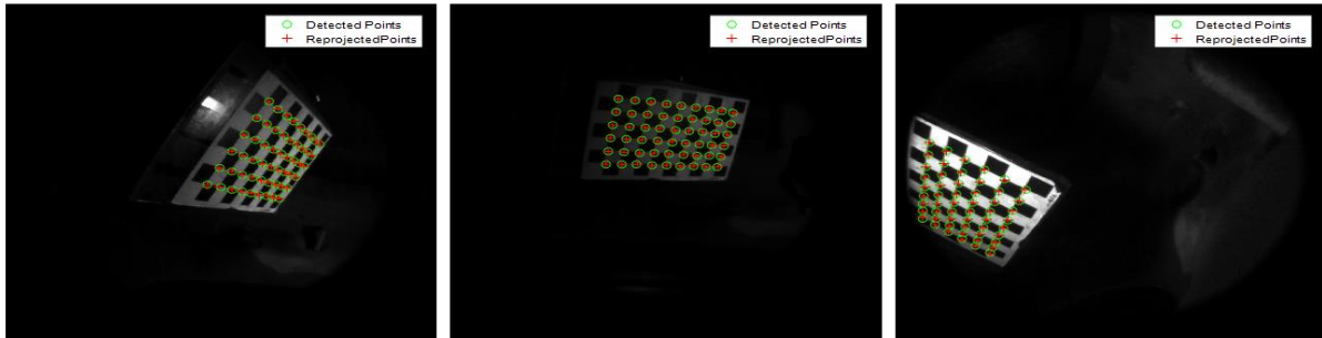
Fig. 4. Example of chess-board target used for calibrating the camera set-up as viewed from the three cameras. Detected calibrations points marked with green circles and reprojected points marked with red crosses.
