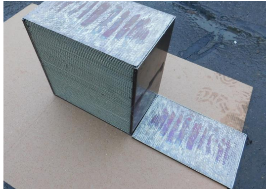
Figure 6: Condition analysis after hot shaker test
