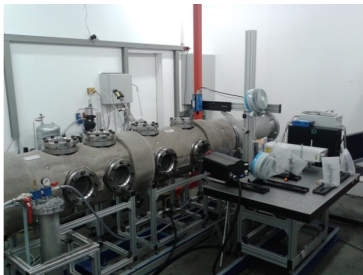
Figure 4 Hot exhaust gas flow rig for investigation of urea injection, evaporation and mixing
