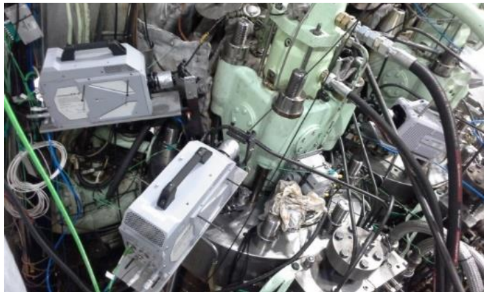
Triple-camera high-speed imaging on two-stroke dual-fuel engine reconstructed 3D flame kernel
