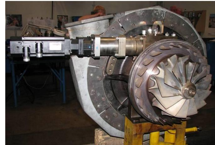
T/C with variable turbine nozzle vanes
