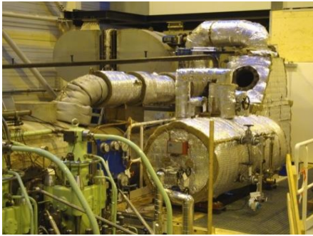
High Pressure Boiler installed on 4T50ME-X
